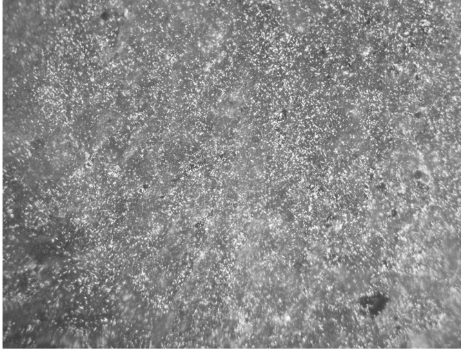
Figure 8. Optical image (10 \times ) of PHB/PEIP blends processed at 170°C for 20 min without catalyst.
